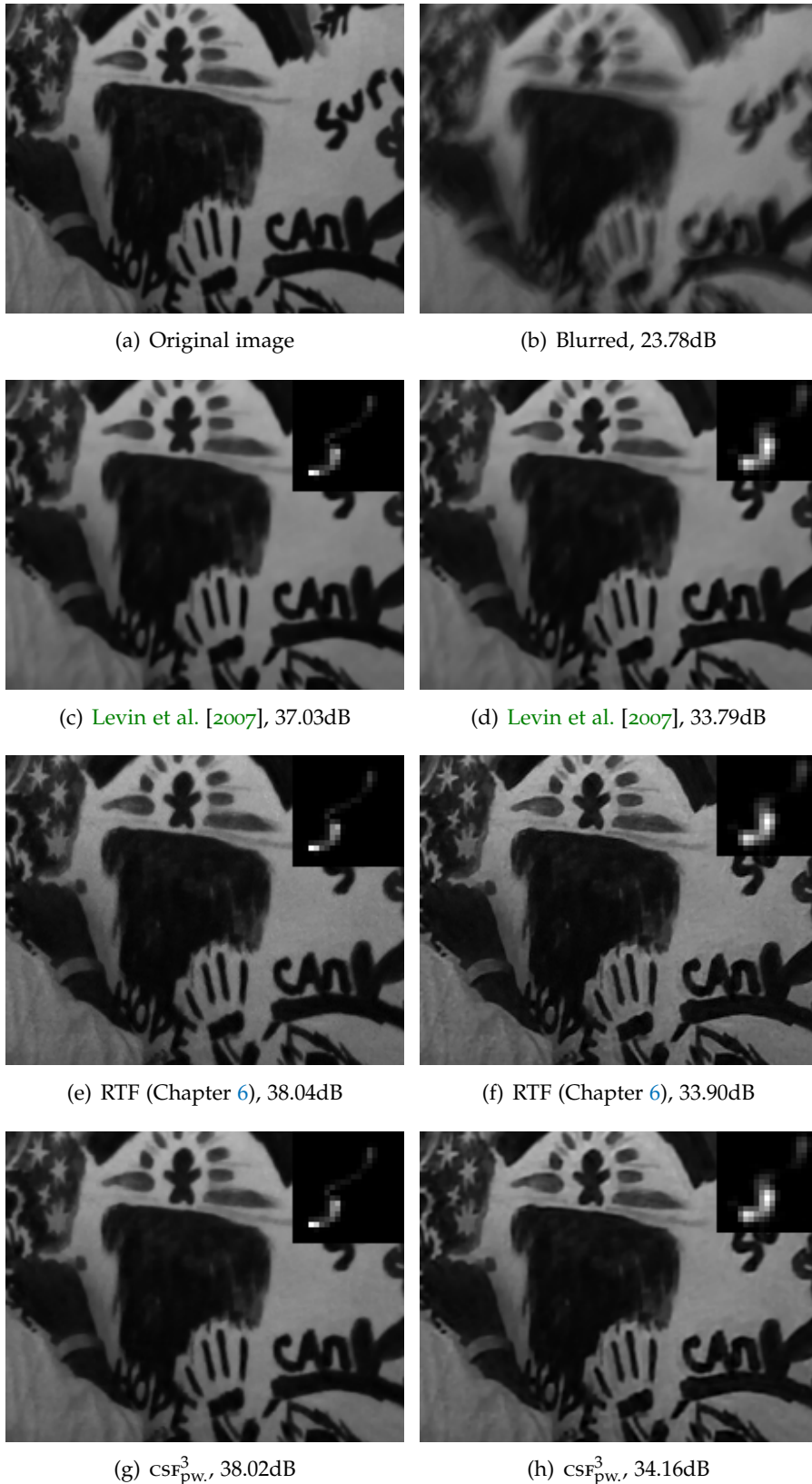
Figure 7.5: Deconvolution example (cropped): Comparison for image deconvolution (cf. Table 7.3) with different blur kernels (ground truth: (c,e,g); estimate via [Levin et al., 2011]: (d,f,h)). Best viewed magnified on screen.
